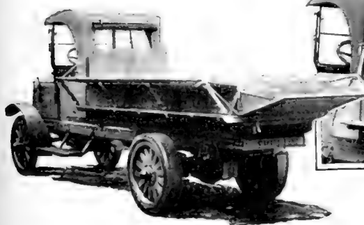
Fig. 5. Extended Flareboard Sides for Carrying Empty Crates, Straw and Other Light Products
